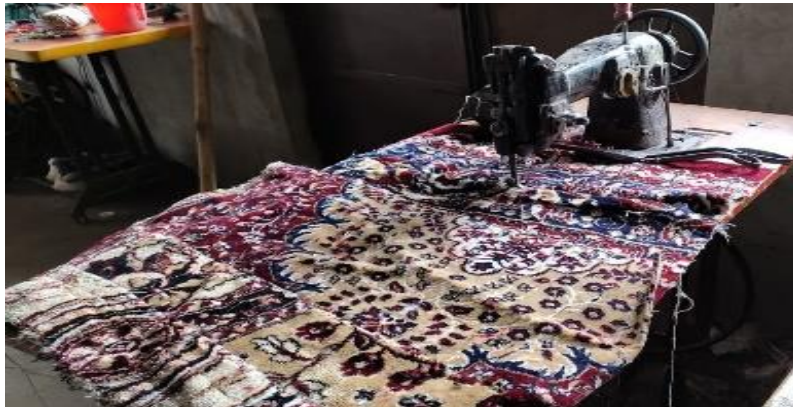
Doormat stitching process with the help of sewing machine.
